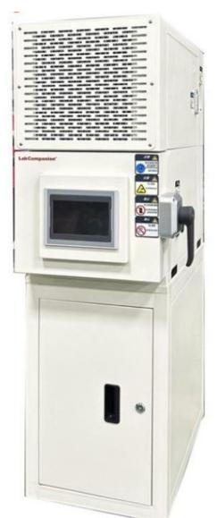
Table type high and low temperature test chamber mainly provides constant temperature and high and low temperature alternating test environment and test conditions for various small industrial products in the research and development, production, inspection and other aspects of the test. It can meet the wide application needs of electronic devices, mobile phone communication, materials and energy, aerospace, colleges and universities, scientific research institutions and other industries.
