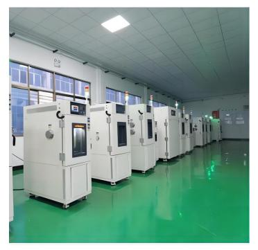
The humidity test can be conducted at the same time as the temperature test, so that the test effect is closer to the natural climate, simulating a worse natural climate, so that the reliability of the tested sample is higher.
